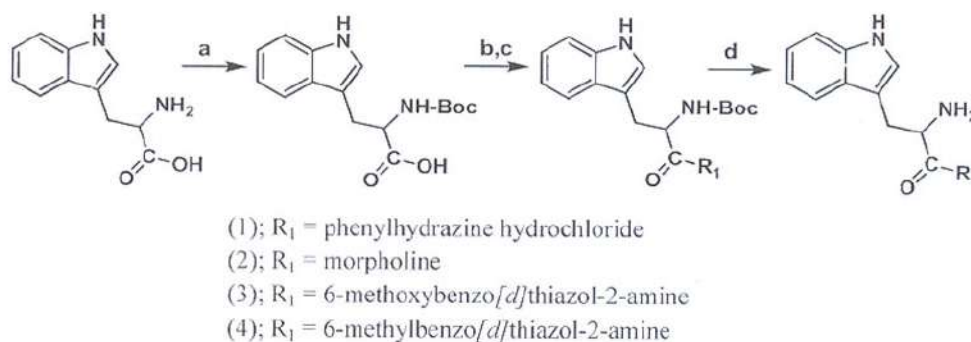
Scheme 3 Synthesis of L (-)-tryptophan amides 26-33 (a) \text{Boc}_2\text{O} , NaOH (aq), THF, \text{H}_2\text{O} , stir overnight, RT; (b) CDI, THF, stir 1 hr, RT; (c) add \text{R}_1\text{NH}_2 , stir overnight, RT; (d) TFA, THF, stir 1 hr., 0^\circ\text{C} .
